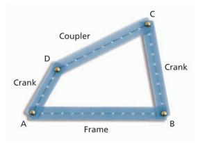
One of the sides is fixed. It is the *frame*. The two sides attached to the frame are the *cranks*. One of the cranks is the driver and the other the follower. The fourth side is called the *coupler*. Quadrilateral linkages are used for windshield wipers, automobile jacks, and reclining lawn chairs.
